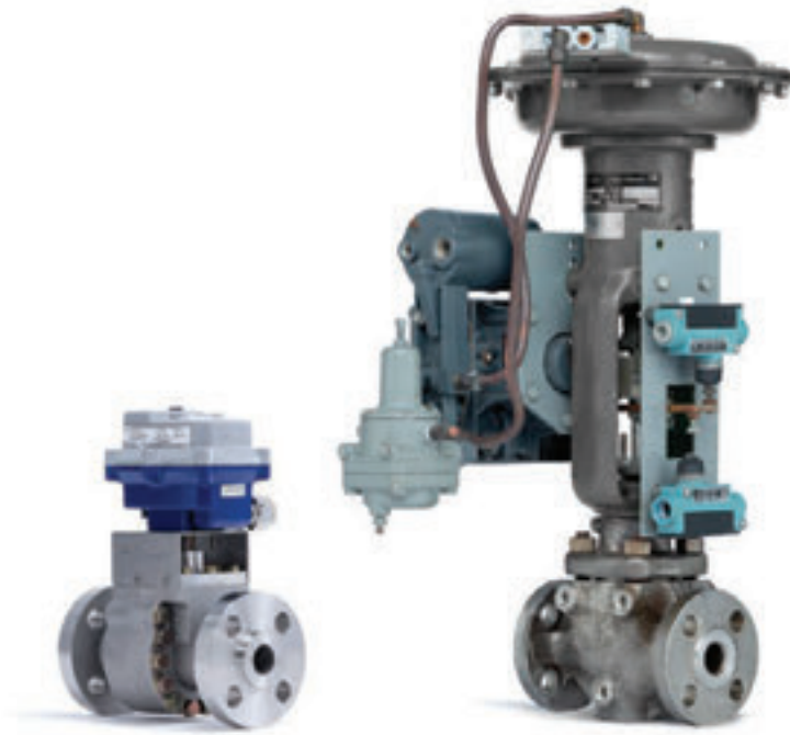
Two ANSI Pressure Class 150 valves, side by side. On the left is the 1" Dilating Disk™ Valve, and on the right is a 1" globe valve. Despite the significant size difference between each valve body and the attached actuators, the Dilating Disk™ Valve delivers equivalent flow rate (Cv) to the globe valve and has been engineered to match the same face-to-face dimensions.
